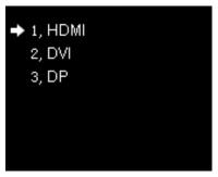
Enter the EDID setting interface of "HDMI" or "DVI" or "DP". Rotate the knob to select conventional resolution; or set width, height and frame rate by knob in the option of "Custom".
