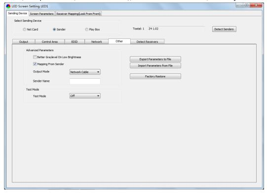
6. **Detect Receivers**: Detect receivers under each net port of Z4 controller, and acquire relevant information about the receivers (Port, Index, Version, Run Time, Support Chips).
