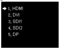
Enter the cropping interface of "HDMI" or "DVI" or "SDI1" or "SDI2" or "DP", press the knob/OK to turn on/off crop. If it has been enabled, set X, Y, width and height of input signal by knob then save the data.
