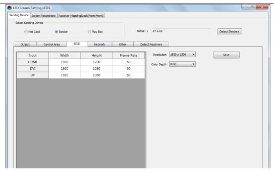
Click the dropdown button to display the resolution list to select the mainstream resolution, and you can also customize the sender resolution, by setting the width/height and frame rate.
