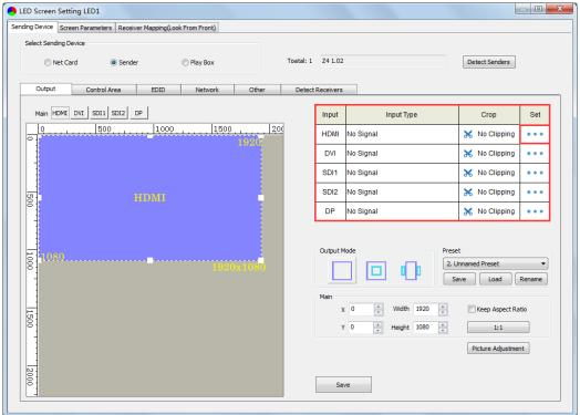
In the clipping interface, check [Crop], and set X, Y, width and height in [Cropping Settings], then click [Save] to complete.
