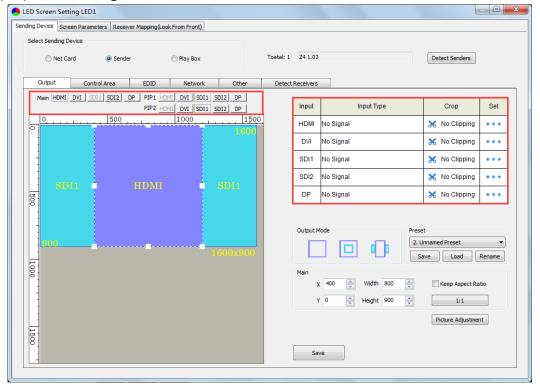
Note: Main and PIP can't select the same source. When PIP1 and PIP2 exist in output mode at the same time, PIP1 and PIP2 can select the same source.
