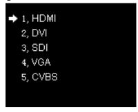
Enter the clip interface of "HDMI" or "DVI" or "SDI" or "VGA" or "CVBS", press the knob/OK to turn on/off clip. Set X, Y, width and height of input signal by knob then save the data.
