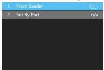
In the submenu, press the knob/OK to turn on or off From Sender. If From Sender is turned on, the sender is set as the connection source. Then select Set by Port to enter the submenu, in which you can choose the Ethernet port from 1 to 20 that needs setting mapping, and set the row offset value(X) and column offset value(Y) of the port, and the width, height, row number, column number and link type of the corresponding cabinets. Finally select Save to save the mapping.
