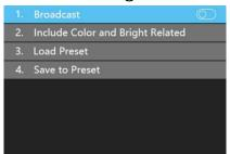
In the submenu, you can press the knob/OK to turn on or off the broadcast function. If Include Color and Bright Related is checked, and you select Save to Preset, then you can save the parameters of the current image that include color and brightness information. You can also select Load Preset and choose an item to load preset parameters.
