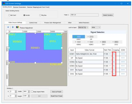
In the cropping setting window, select the **Enable** check box, and set the row starting point (X), the column starting point (Y), and the width and height in the **Cropping Settings** area.
