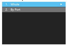
Output shift includes two selections: Whole and By Port. On the submenu of Whole, you can rotate the knob to set the row starting point (X) and column starting point (Y) of the whole image and save the setting; on the submenu of By Port, you can respectively set the row starting point (X) and column starting point (Y) of the image of the 20 Ethernet ports and save the setting.
