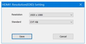
Click the dropdown button. From the resolution list, you can select a conventional resolution, or select **Custom** and set the width, height, frame rate and standard of the customized resolution.
