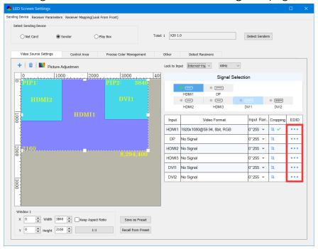
In the **Resolution (EDID) Setting** dialog box, the resolution of the current sender is displayed by default.
