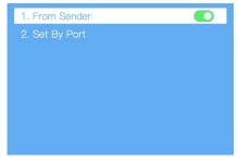
In the submenu, press the knob/OK to set the sender as the connection source. Then select **Set by Port** to enter the submenu, in which you can choose the Ethernet port from 1 to 16 that needs setting mapping, and set the row offset value(X) and column offset value(Y) of the port, and the width, height, row number, column number and link type of the corresponding cabinets. Finally select **Save** to save the mapping.
