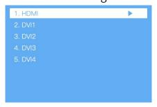
In the EDID setting submenu of **HDMI** and **DVI1/2/3/4** (take **HDMI** as an example), you can rotate the knob and select a conventional resolution to save the selected resolution to the sender, or select **Custom** and rotate the knob to adjust the width, height and frame rate, and then select **Save** to save the setting in the sender.
