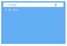
Output shift includes two selections: Whole and By Port. On the submenu of Whole, you can rotate the knob to set the row starting point (X) and column starting point (Y) of the whole image and save the setting; On the submenu of By Port, you can respectively set the row starting point (X) and column starting point (Y) of the image of the 16 Ethernet ports and save the setting.
