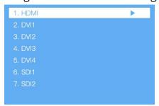
In the cropping setting submenu of HDMI or DVI1/2/3/4 or SDI1/2, press the knob/OK to turn the cropping function on or off. If Enable has been switched on, you can rotate the knob to set the row starting point (X), the column starting point (Y), and the width and height of the signal image, and then select Save.
