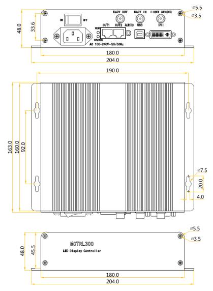
Tolerance: ±0.3 Unit: mm
