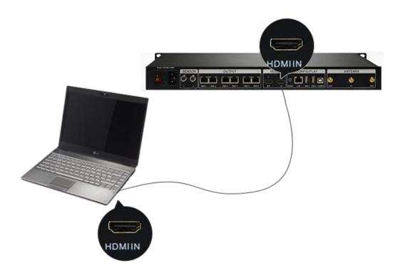
**Note:** The C7 will automatically switch to play the sync signal program when an external HDMI signal input is detected. You can press the **[Input Switch]** button to return to async signal program playing.
