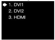
In the EDID setting submenu of **HDMI** or **DVI**, you can rotate the knob and select a conventional resolution to save the selected resolution to the sender, or select **Custom** and set the width, height and frame rate, and then select **Save** to save the setting to the sender.
