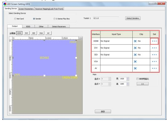
In the clipping interface, check [Clipping], and set X, Y, width and height in [Clipping Information], then click [Save] to complete.
