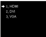
Enter the EDID setting interface of "HDMI" or "DVI" or "VGA". Rotate the knob to select conventional resolution; or set width, height and frame rate by knob in the option of "Custom".
