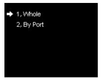
Output shift includes two ways: "Whole" and "By Port". In the setting interface of "Whole", you can rotate the knob to set X and Y of the whole image and save it; in the setting interface of "By Port", you can set X and Y of the image of each net port respectively, then save it.
