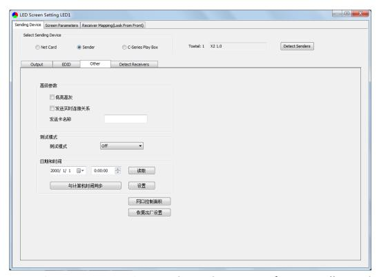
4, **Detect Receivers**: Detect receivers under each net port of X2 controller, and acquire relevant information about the receivers (Port, Index, Version, Run Time, Support Chips).
