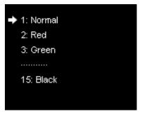
© Video Change: Enter the setting interface of "Video Change", and press the knob/OK to turn on/off the option of "By Take". If "By Take" is in the closed status, you can directly press the selection key of video source to switch the playing video; if "By Take" has been turned on, you must continue pressing "Take" to switch the playing video after pressing the selection key of video source.
