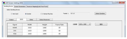
Click the dropdown button to display the resolution list to select the mainstream resolution, and you can also customize the sender resolution, by setting the
