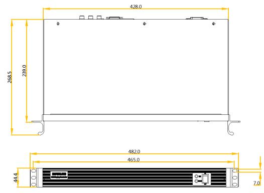
Tolerance: ±0.3 Unit: mm
