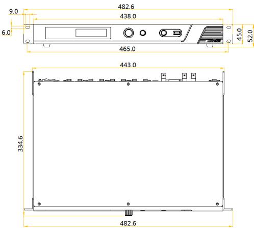
Tolerance: ±0.3 Unit: mm
