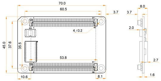
Tolerance: ±0.3 Unit: mm
